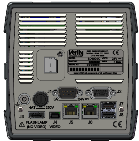
J2 コネクタ DIO & RS232 & Synchronization (J2 is HD15 with internal sockets)
